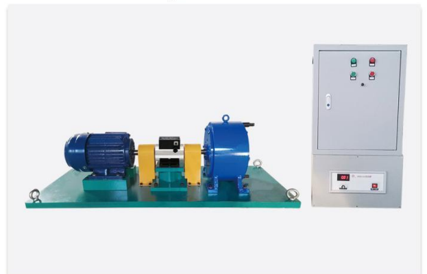
永磁同步电机加载测试台 Permanent magnet synchronous motor loading test bench
