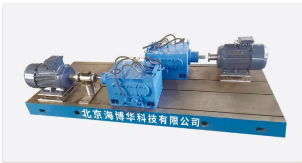
电机对拖式变速箱模拟加载测试台 Motor to drag transmission simulation loading test bench
