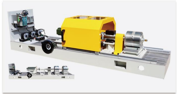
永磁同步电机加载测试台 Permanent magnet synchronous motor loading test bench
